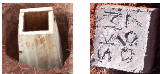
Plate 3.2: Model of Short Truncated Pillar and Monumented new control pillar (SKW 007) at Vuga market.
